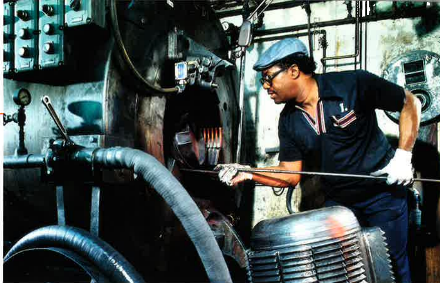
Cold isostatic pressing, shown here, utilizes pressures in excess of 30,000 psi to mold the powdered tungsten into a preform.
